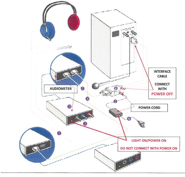
IS OFF PRIOR TO CONNECTING OR DISCONNECTING THE INTERFACE CABLE TO/FROM THE COMPUTER
